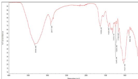
Figure 4: FTIR spectra of cotton fabric (inorganic PCM)
