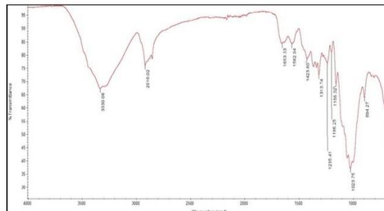
Figure 5: FTIR spectra of control cotton fabric
