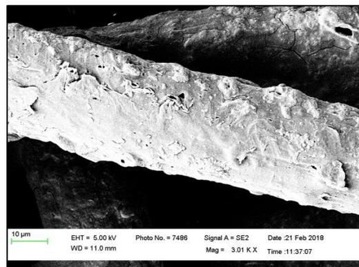
Figure 2: Morphology of the microcapsule-treated fabrics - SEM
