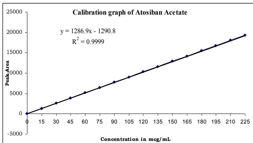
Figure 3: Calibration curve of the Atosiban Acetate by RP-HPLC
